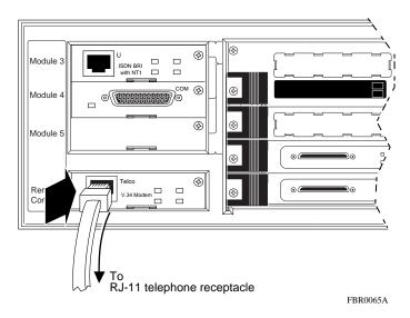
Figure 2-1. Passport 5430 V.34 Modem Adapter Module Connector
